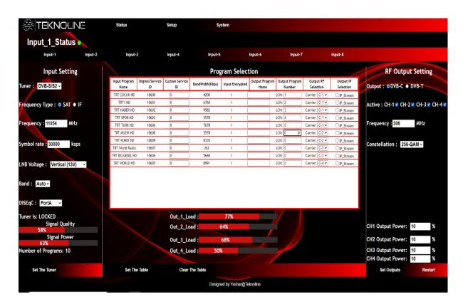
Output modulation type and channel can be selected from the OUTPUT RF Selection section.
